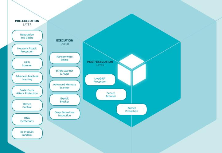
These are some of ESET's core technologies, showing approximately when and where they can detect and/ or block a threat during its lifecycle in the system.
